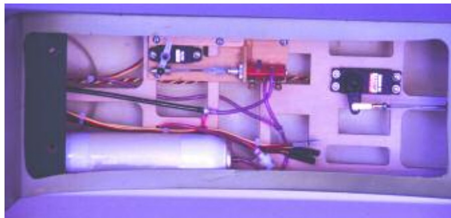
The fuselage provides plenty of room to mount radio and retract equipment.
